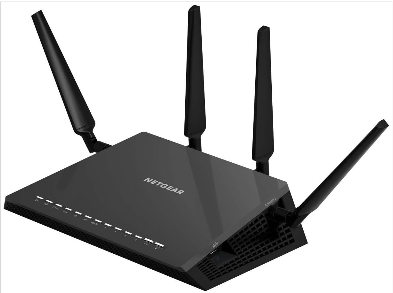
Image: Front and side view of the NETGEAR Nighthawk X4S R7800 router, showing its four external antennas and front panel indicator lights.
