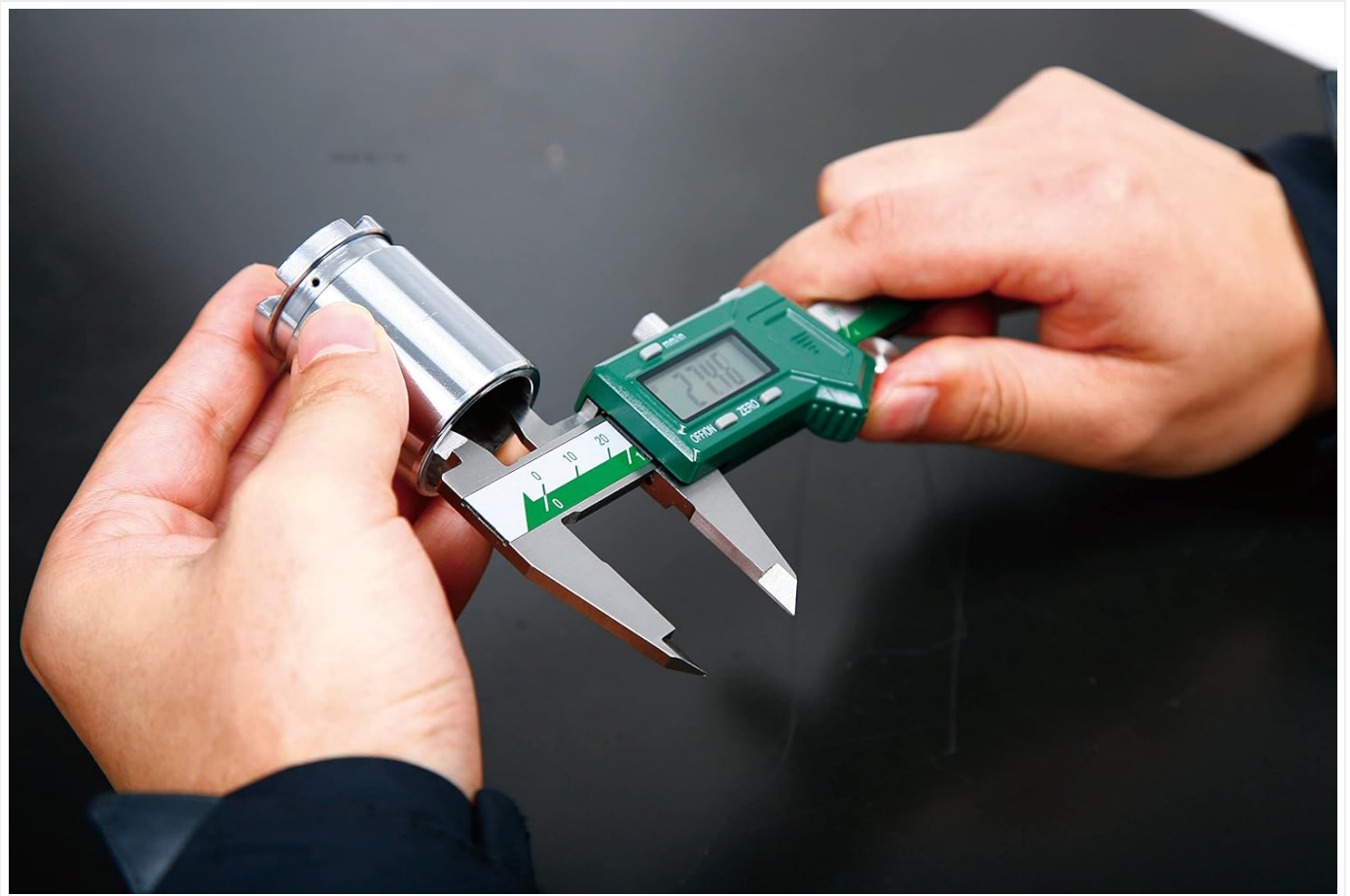
Figure 6: A user demonstrating the measurement of an external diameter on a cylindrical metal part using the INSIZE 1108-150 Electronic Caliper.
