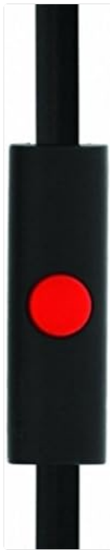
Image 4: The in-line control button for call and music management.
