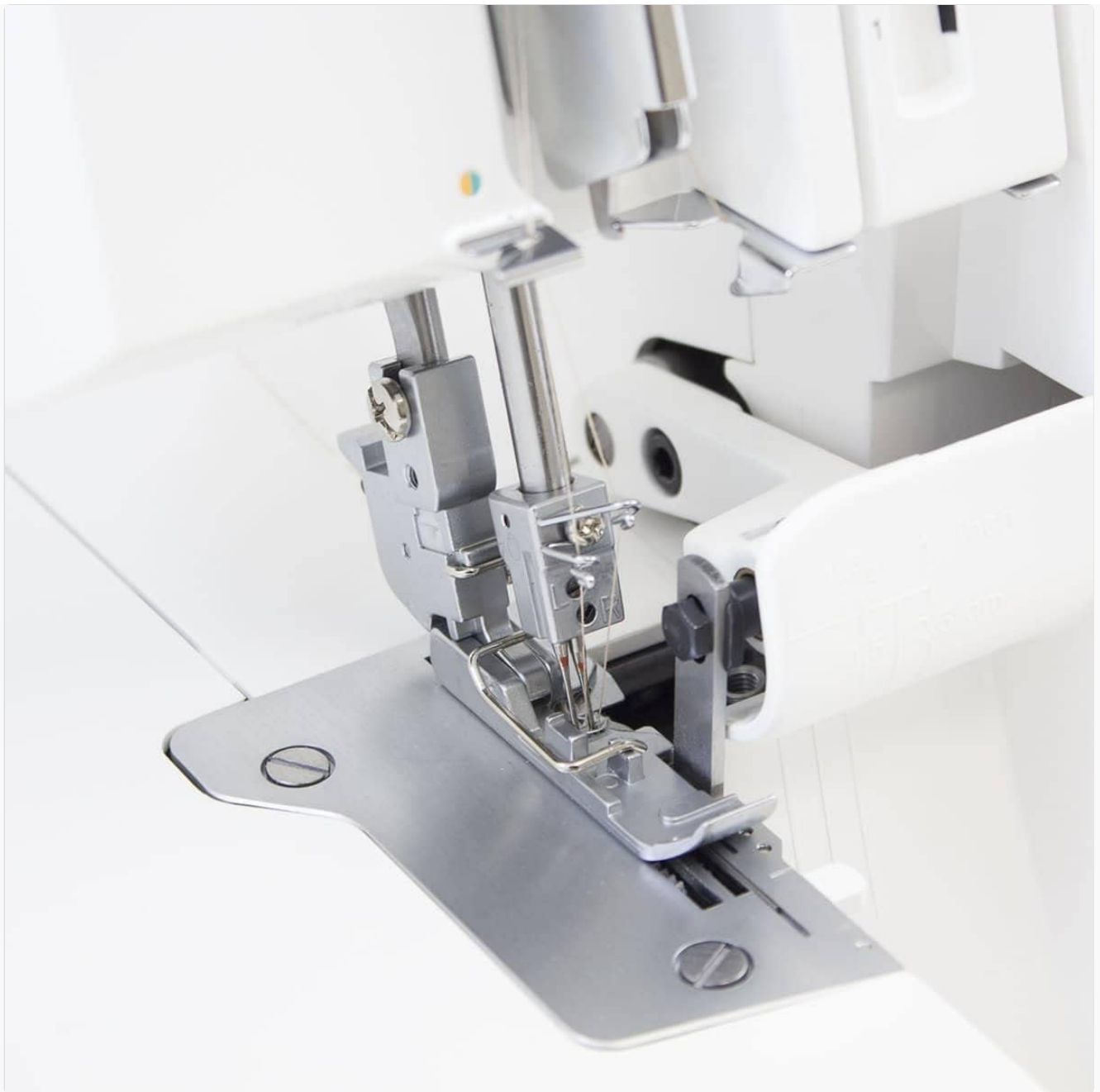
Figure 4.3: Detailed view of the needle and presser foot area on the Juki MO-104D, highlighting the working space.
