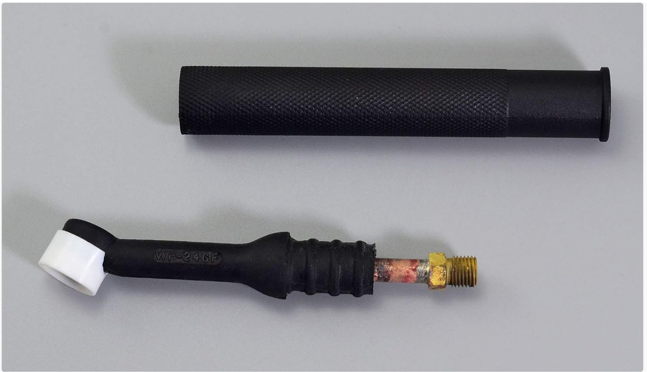
Figure 3.4: Disassembled view of the torch head, showing the internal components and handle.
