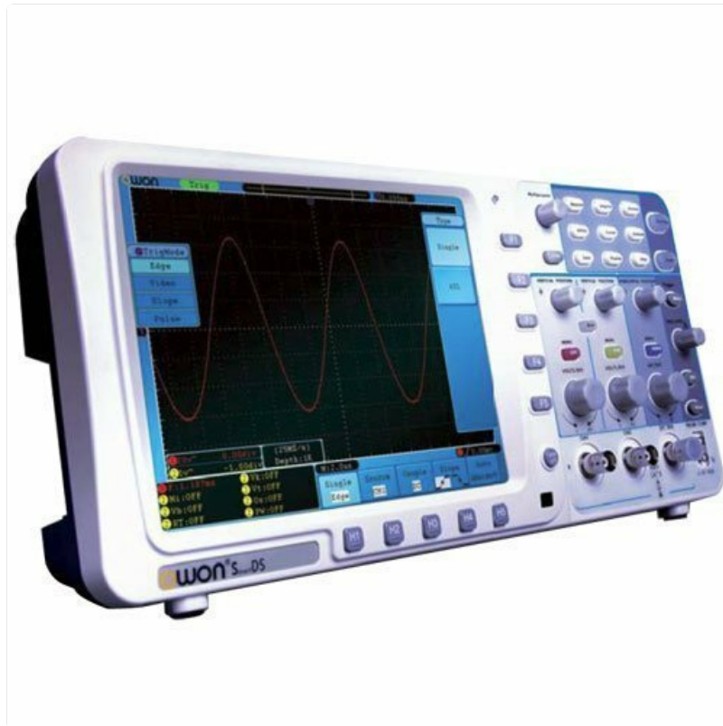
Figure 4.1: Front view of the OWON SDS6062 Digital Storage Oscilloscope, showing the display, control knobs, and function buttons.
