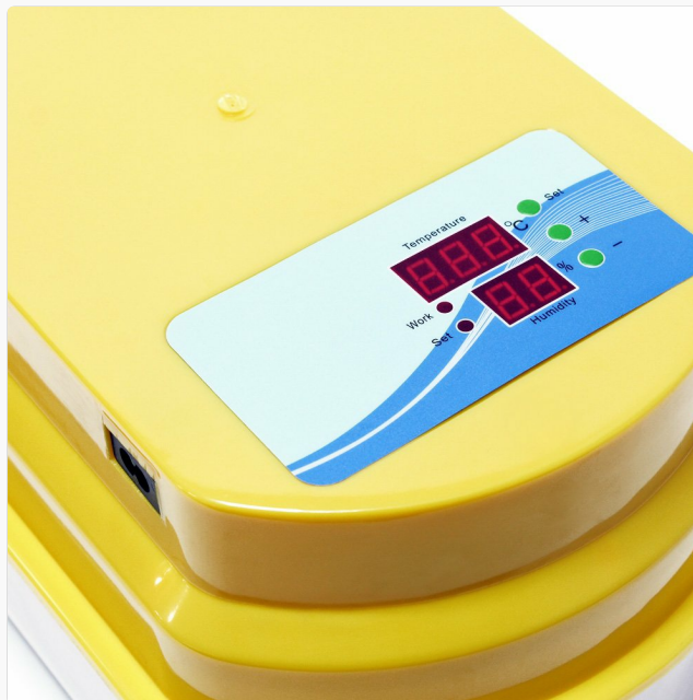
Figure 3.4: Close-up of the control panel, displaying LED indicators for temperature and humidity, along with 'Set' and adjustment buttons.
