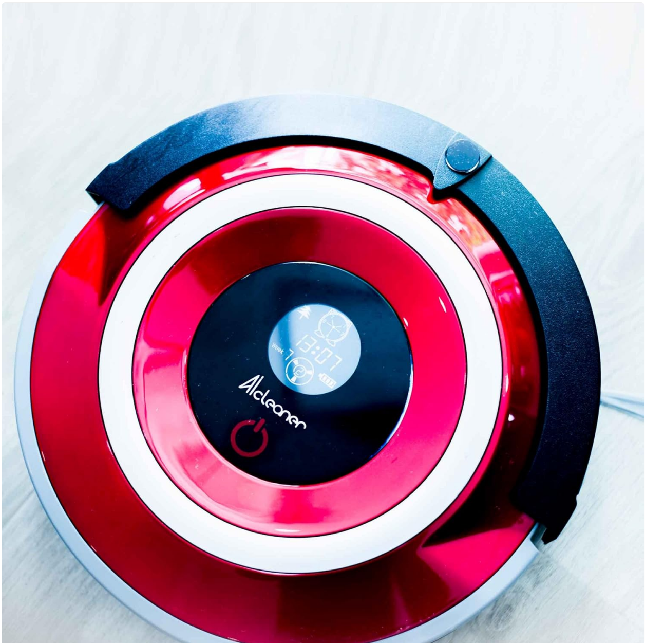
Image 2.1: Top view of the Tango Aicleaner Plus, showing the control panel and display. This display indicates charging status and operational modes.
