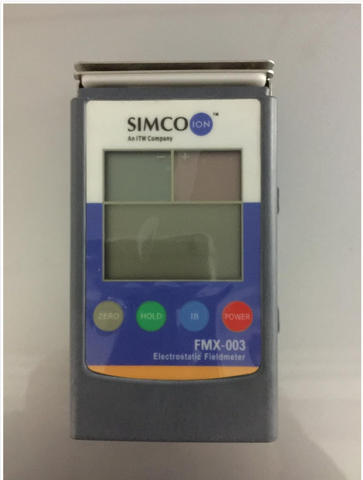
Figure 2: A clear front view of the FMX-003 meter, highlighting the display and control buttons: ZERO, HOLD, IB (Ion Balance), and POWER.
