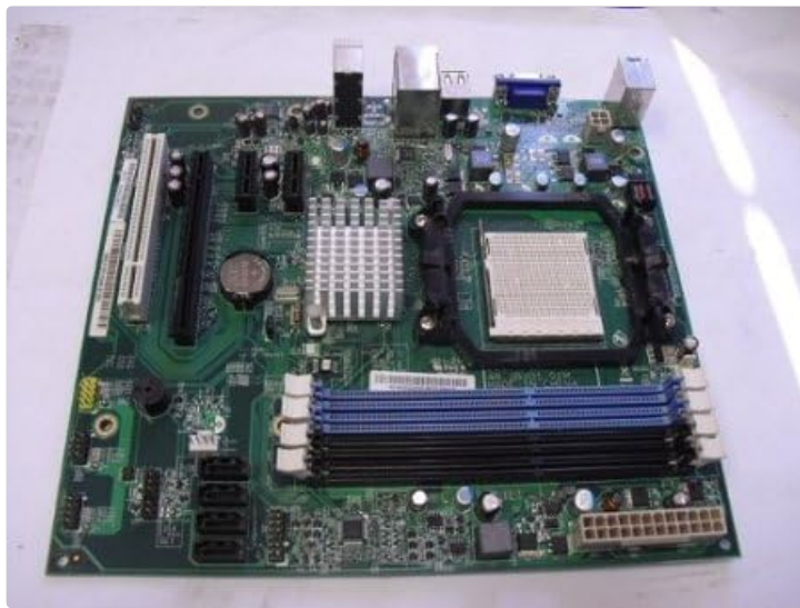
Figure 1: Top-down view of the eMachines ET1352-01 Desktop Motherboard. This image displays the various components including the CPU socket, RAM slots, expansion slots, and I/O ports.
