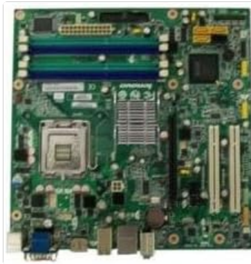
Figure 1: eMachines ECS 945GCT-M3 Desktop Motherboard. This image displays the main components including the CPU socket, memory slots, expansion slots, and various ports.
