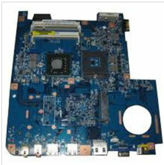
Image: eMachines D525 Intel Laptop Motherboard (MB.N4501.002). This image displays the overall layout of the motherboard, including various connectors and component placements.
