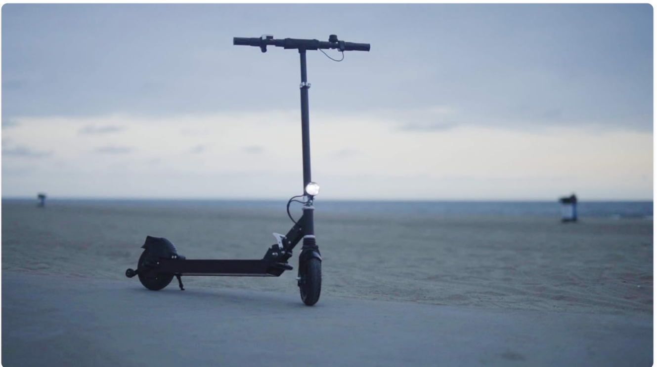
Figure 3: The Glion Dolly in its vertical self-standing folded position.
