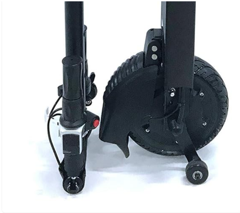
Figure 2: The Glion Dolly in its folded, dolly-mode, allowing it to be rolled like luggage.
