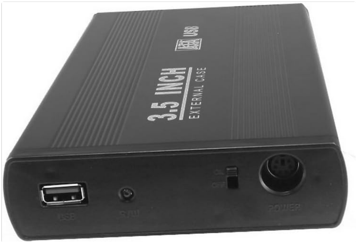
Image: The rear panel of the enclosure, featuring the USB port, DC 12V power input, and power ON/OFF switch.
