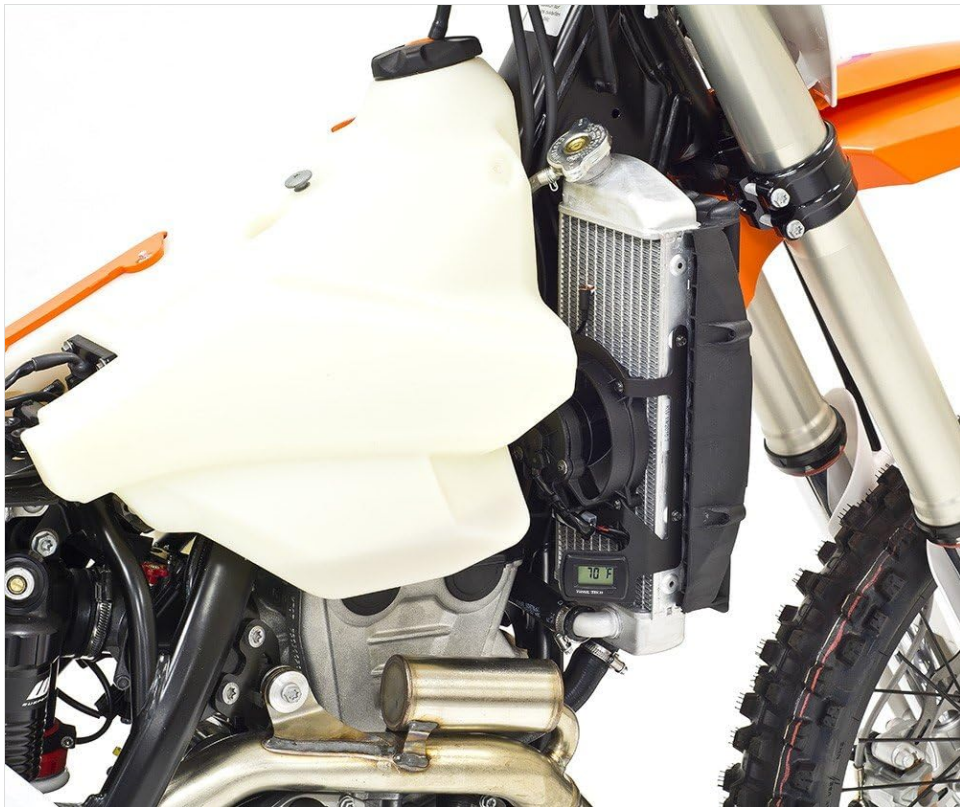
Image 1: Close-up of the digital fan kit installed on the radiator, with the digital temperature display visible.
