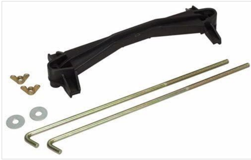
Image: All components of the Aftermarket Battery Hold Down Kit 50149. This includes the main black plastic clamp, two long metal J-hook bolts, two small metal wing nuts, and two flat metal washers.
