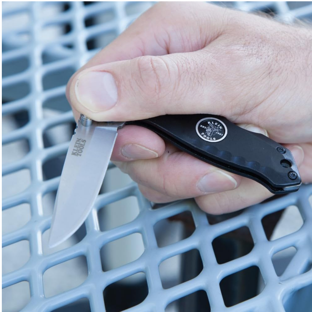
Figure 2: Proper grip and thumb placement for opening the knife blade.
