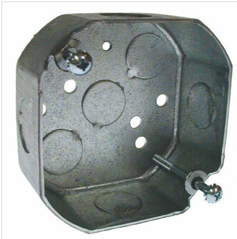
Figure 1: RACO 296 4-Inch by 1-1/2-Inch Deep Ceiling Fan Support Box. This image displays the RACO 296 ceiling fan support box, a galvanized steel octagonal electrical box designed for securely mounting ceiling fans and light fixtures. It features multiple knockouts for wiring entry and two pre-installed screws for fixture attachment.
