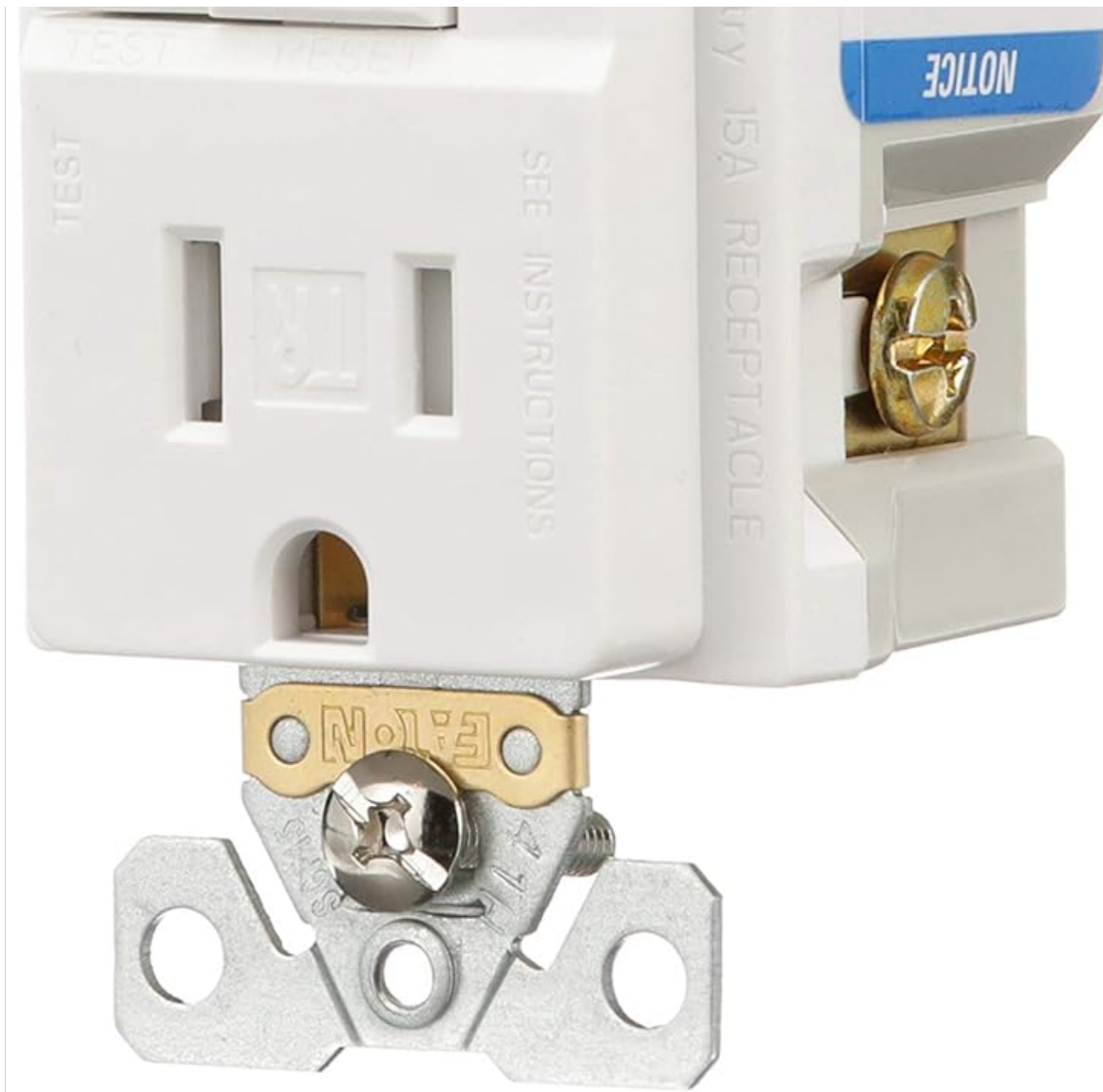
Image: Side profile of the Eaton TRSGF15W GFCI receptacle. This view highlights the side wiring terminals and includes a blue "NOTICE" sticker indicating that the device is not intended for use in wet and damp locations as defined by 2008 NEC 406.8 requirements, reinforcing its indoor-only application.
