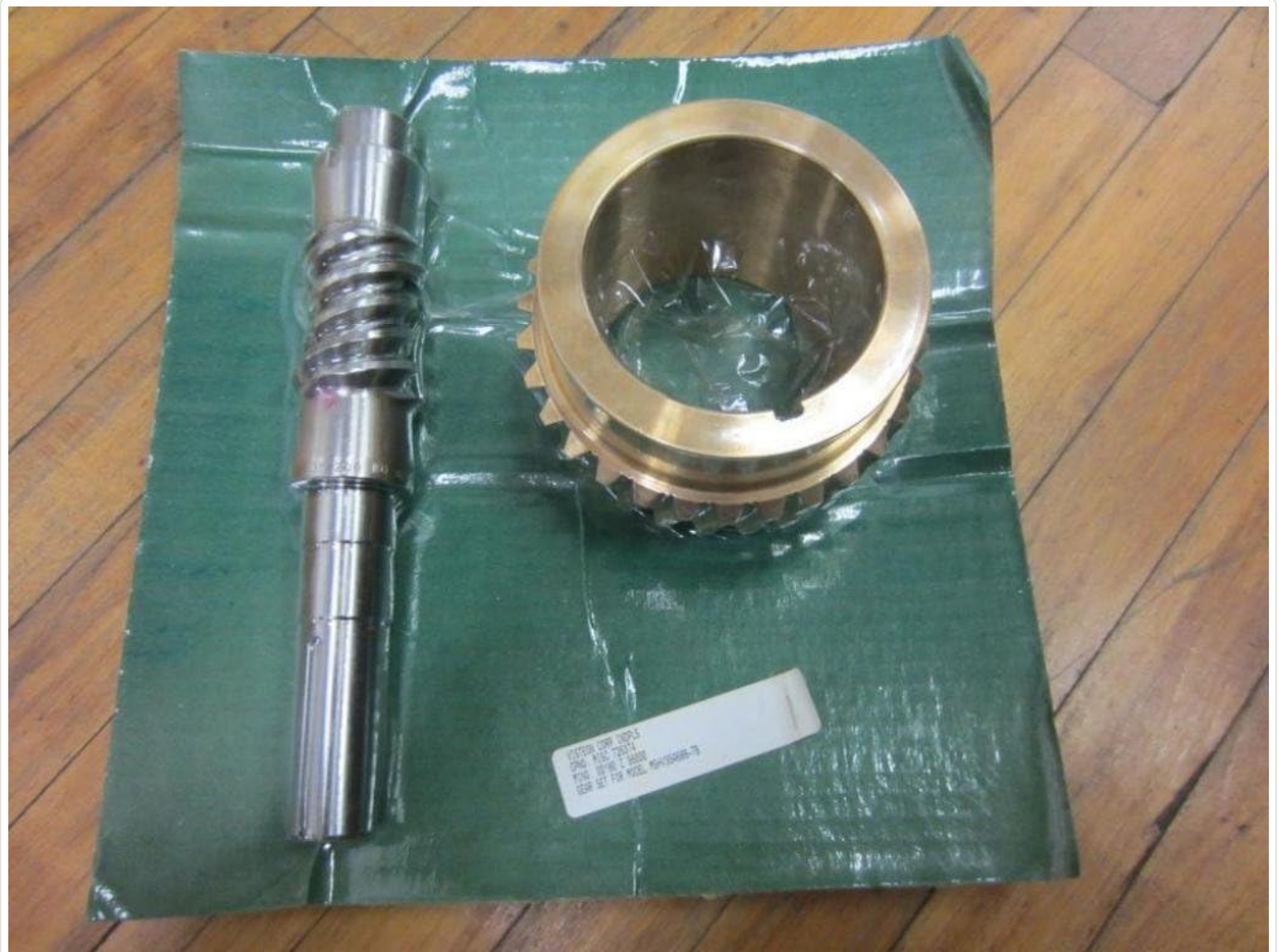
Figure 2.2: The worm gear and its corresponding ring gear, which are critical components for power transmission within the speed reducer.
