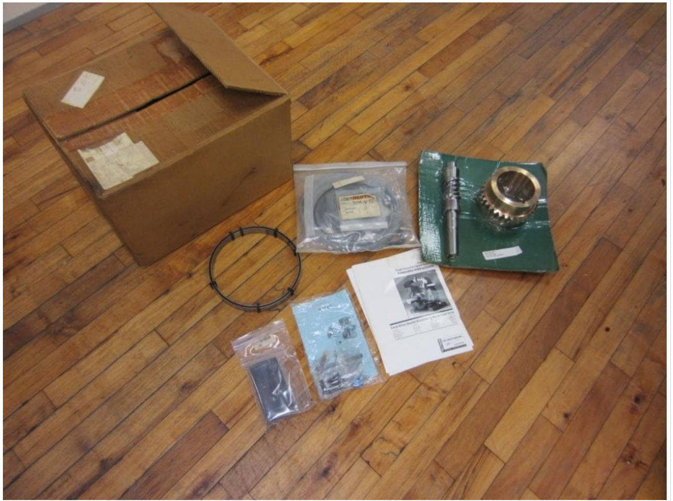
Figure 2.1: Overview of the Visteon MSHV35A688-7B Gear Set Rebuild Kit contents, including the main gear components, bearing kit, and instruction manuals.
