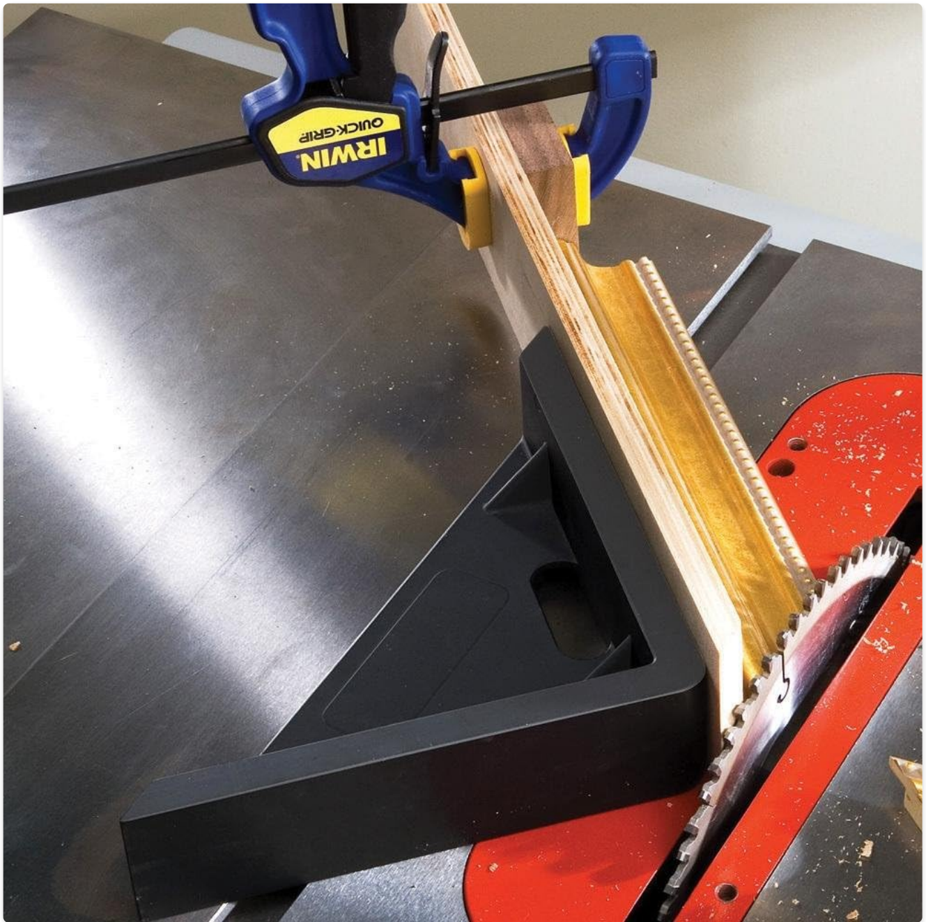
Figure 3: Demonstrates how a workpiece can be clamped to the sled for secure cutting.
