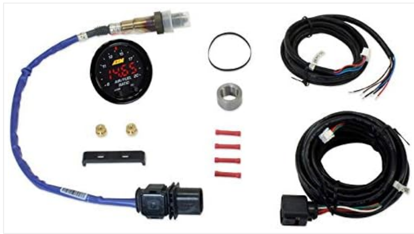
Image 5.2: The wideband sensor and associated wiring harnesses. Proper connection of these components is essential for accurate AFR readings and data output.
