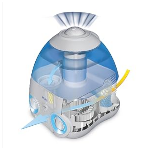
Image 4.1: An internal diagram illustrating how a cool mist humidifier operates, showing water being wicked up by the filter and air passing through to create mist.
