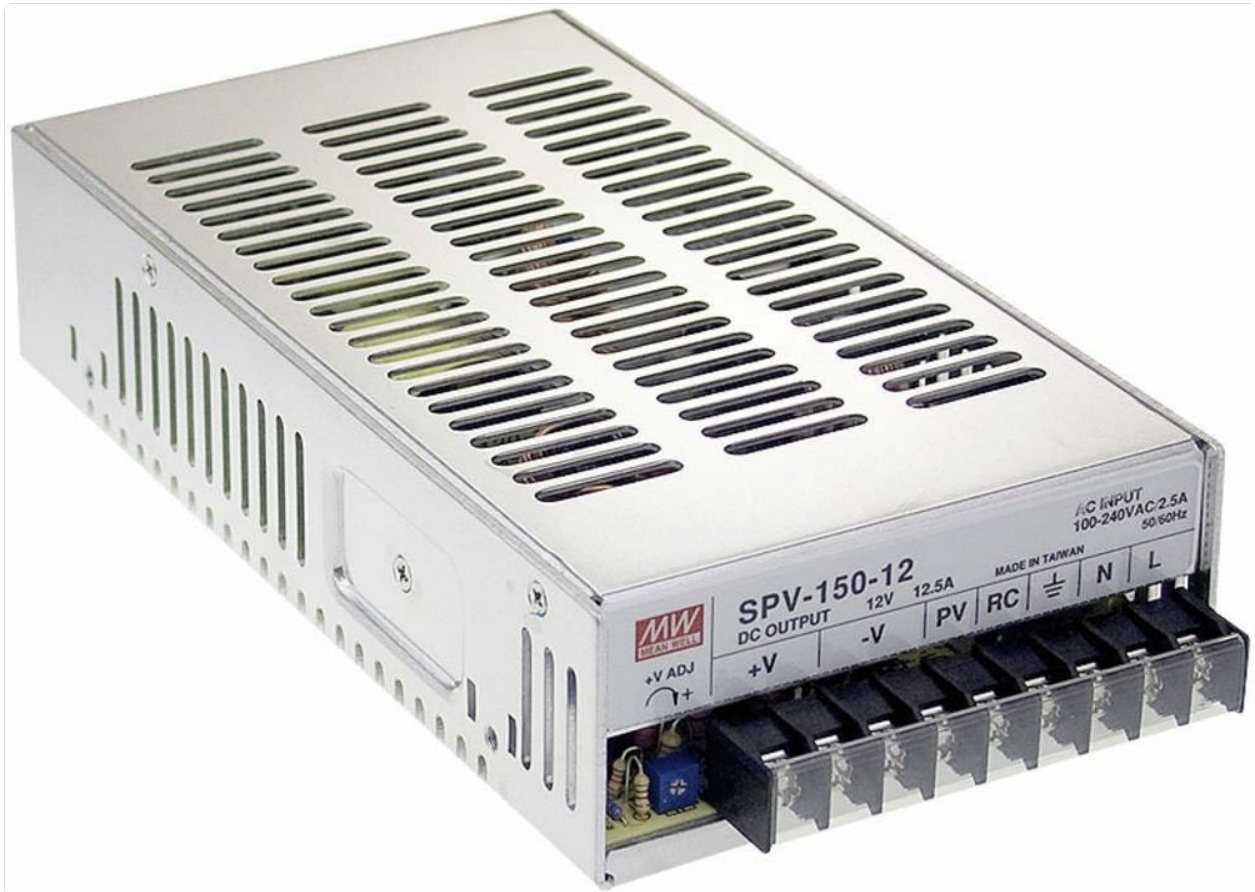
Figure 1: MEAN WELL SPV-150 Series Power Supply. This image displays the AC input terminals (N, L, Ground), DC output terminals (+V, -V), and the +V ADJ potentiometer for fine-tuning the output voltage. The label indicates a 12V, 12.5A output, but the SPV-150-24 model provides 24V, 6.25A.
