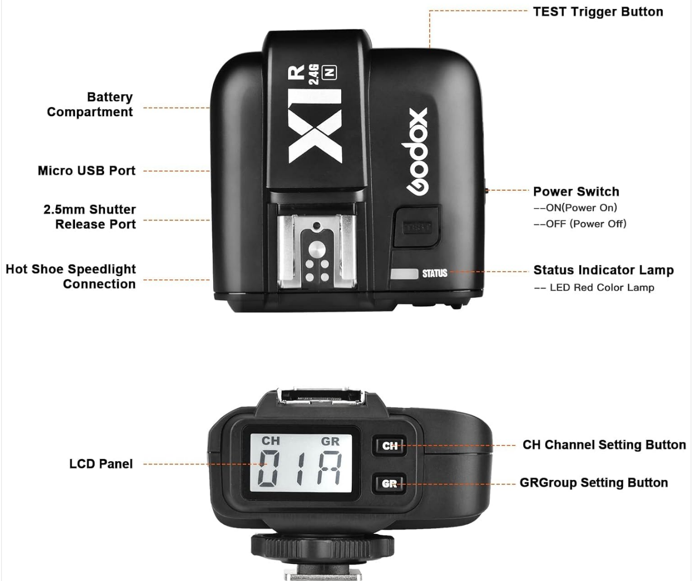
Figure 1: Godox X1R-N Receiver with labeled components.
