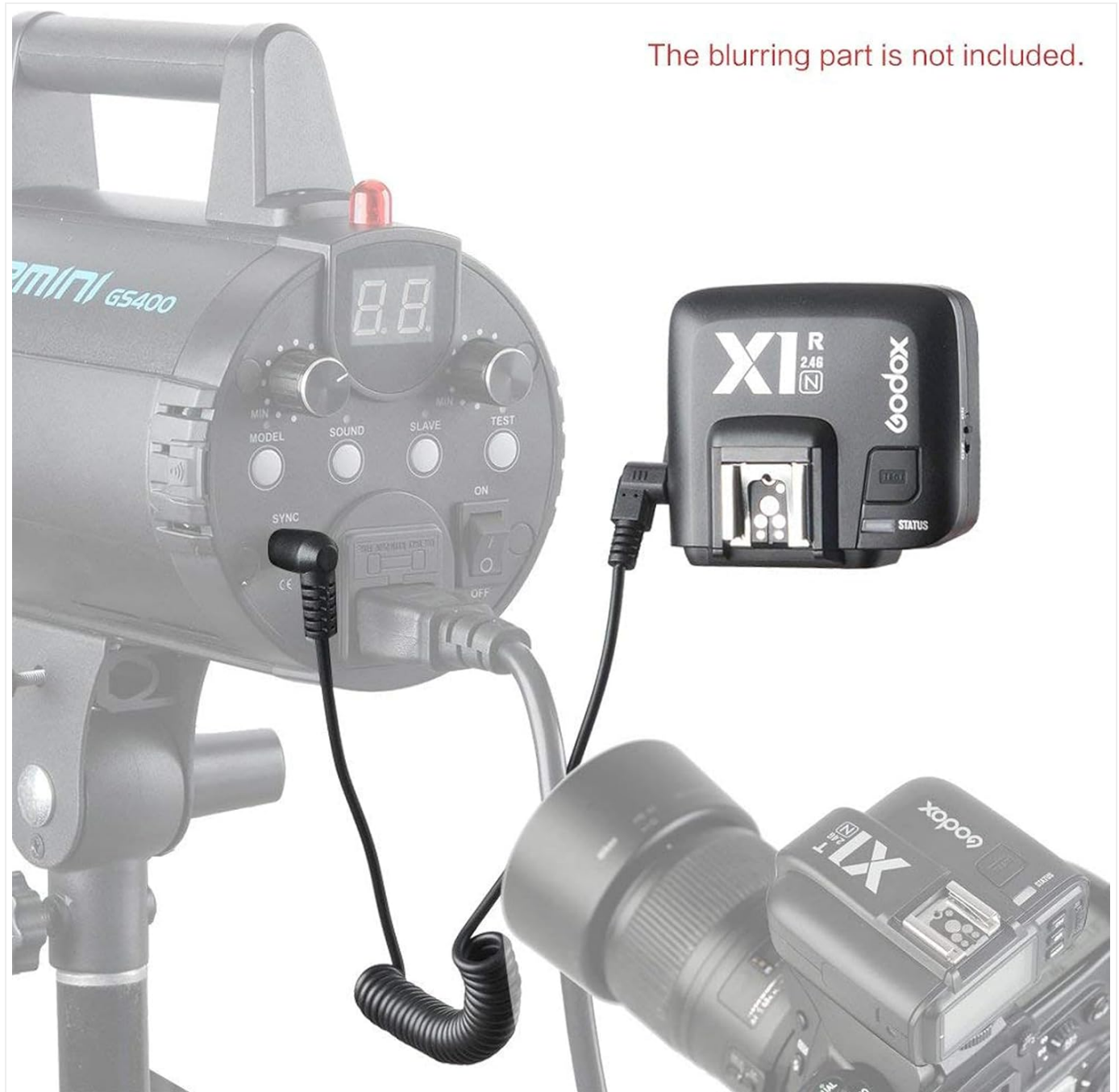
Figure 4: Connecting the X1R-N receiver to a studio flash.
