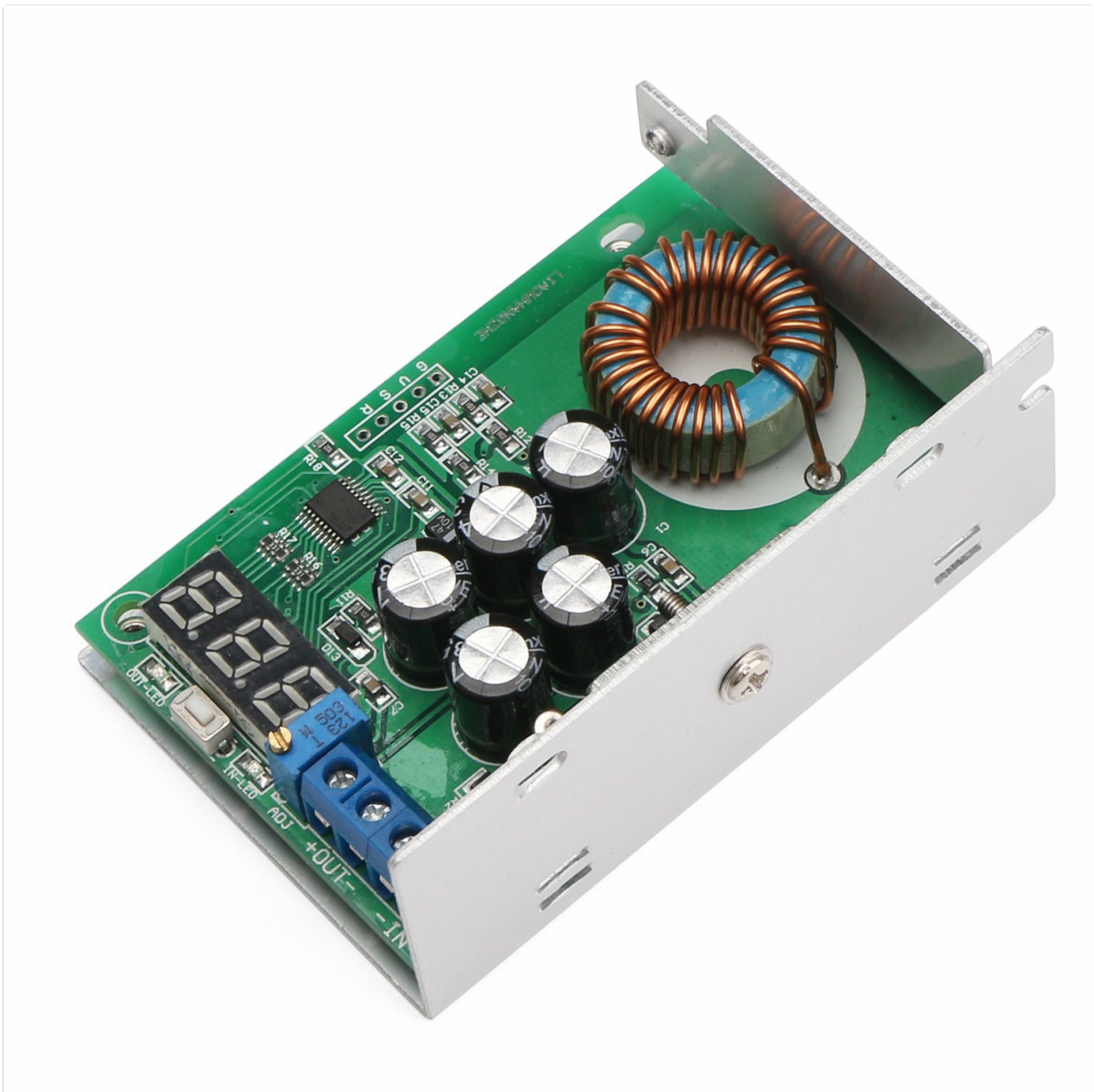
Image 2: Top-down view of the module, showcasing the main components including the large inductor, electrolytic capacitors, and the PCB with integrated circuits. The metal casing is partially visible.
