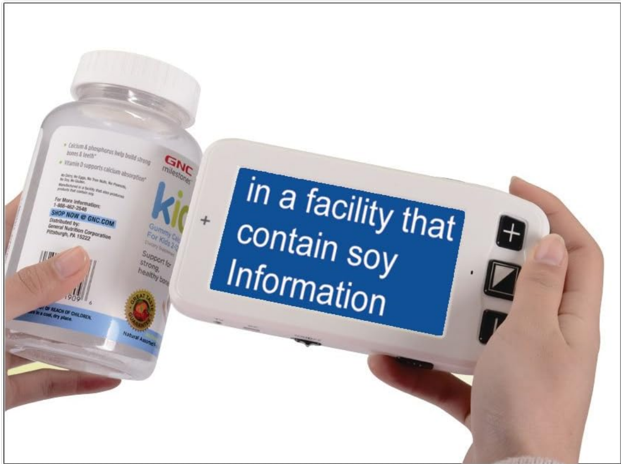
Figure 2: The magnifier in use, demonstrating its ability to enlarge text for easier reading.
