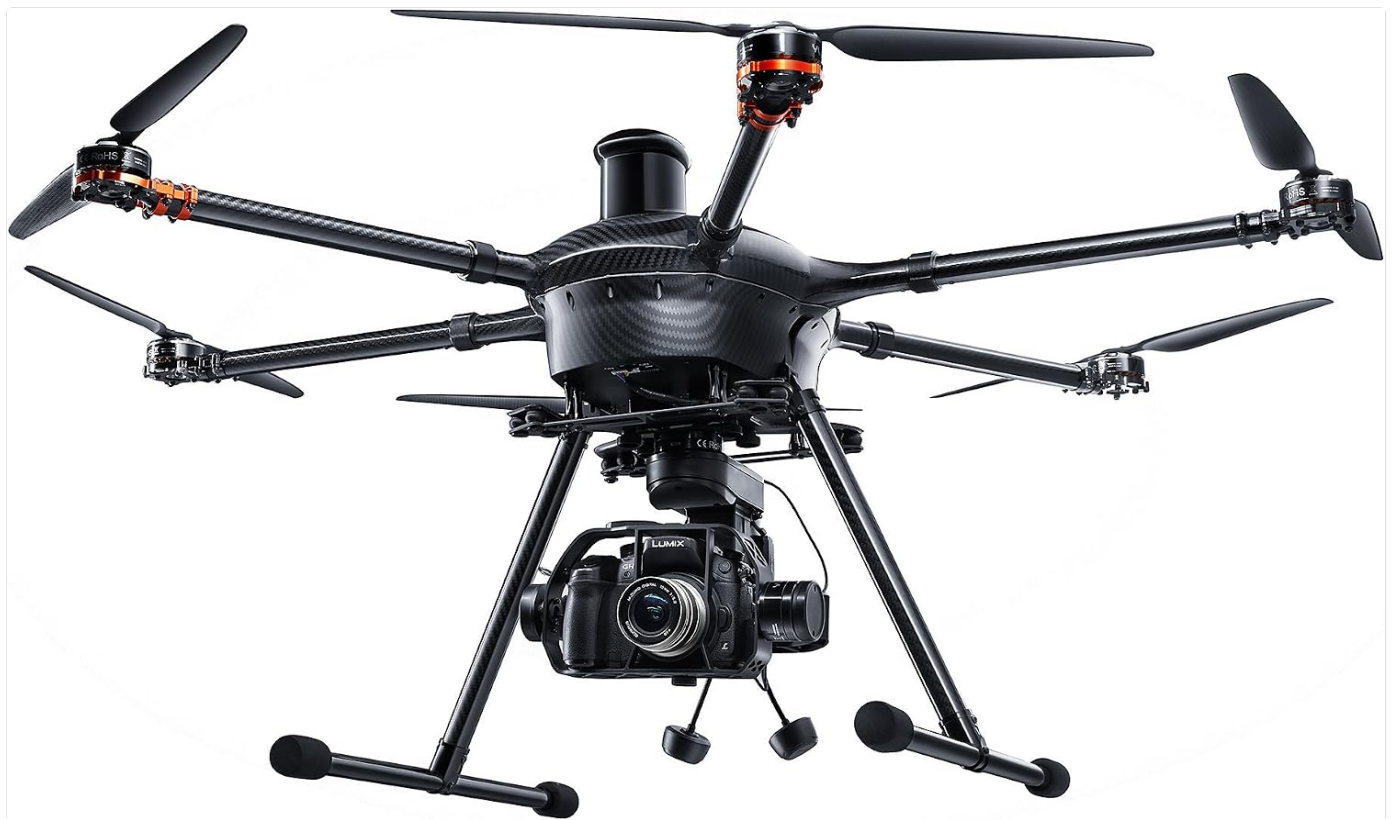
Figure 2.1: Front view of the Yuneec Tornado H920 Hexa-Copter with a camera and gimbal attached, showing its six propellers and retractable landing gear.
