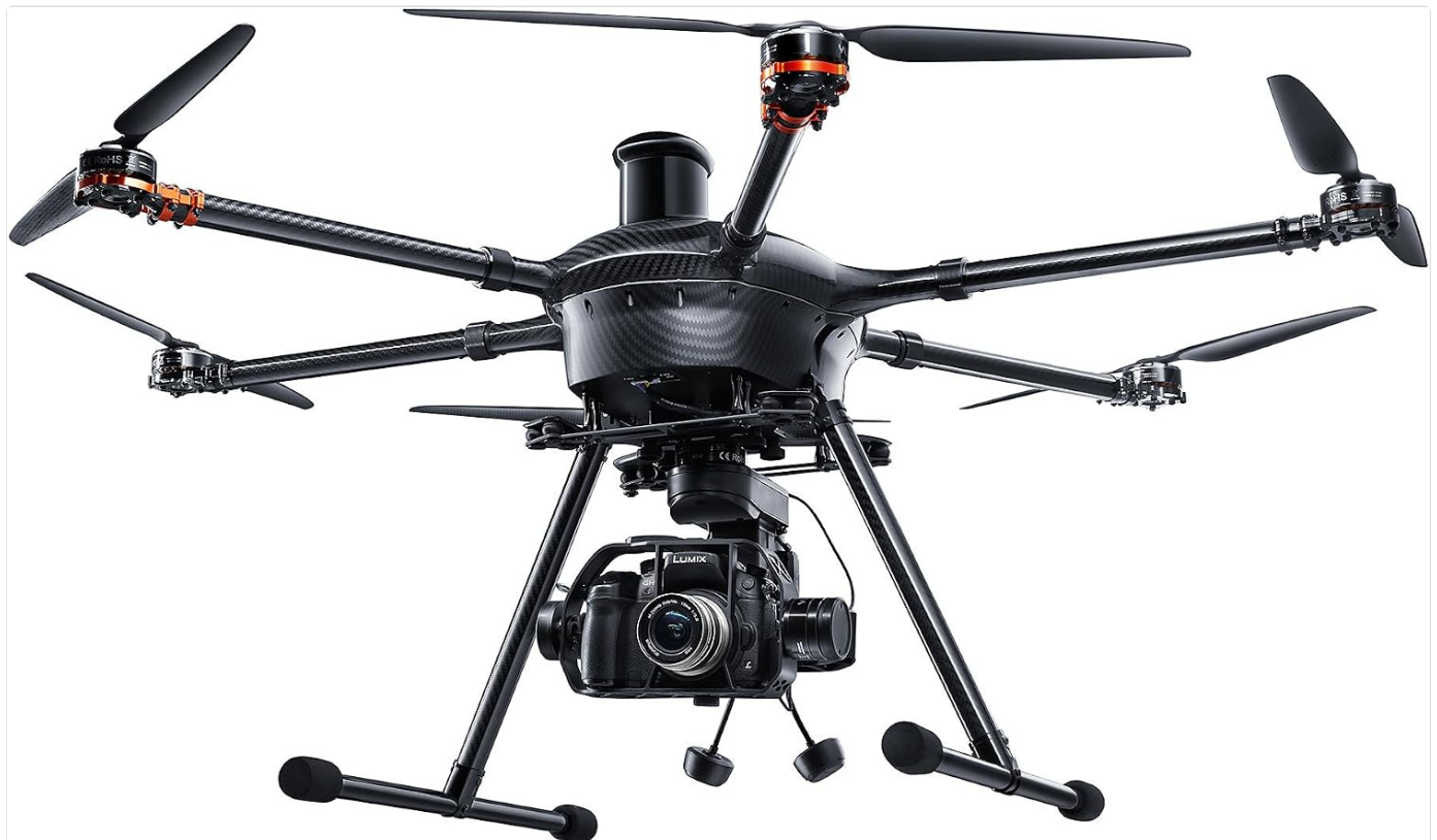
Figure 2.3: The Tornado H920 with its landing gear in the retracted position, demonstrating the clear view for the camera.
