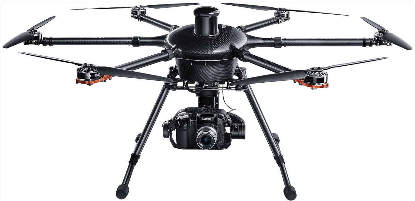
Figure 2.2: Another perspective of the Tornado H920, highlighting its carbon fiber frame and motor mounts.
