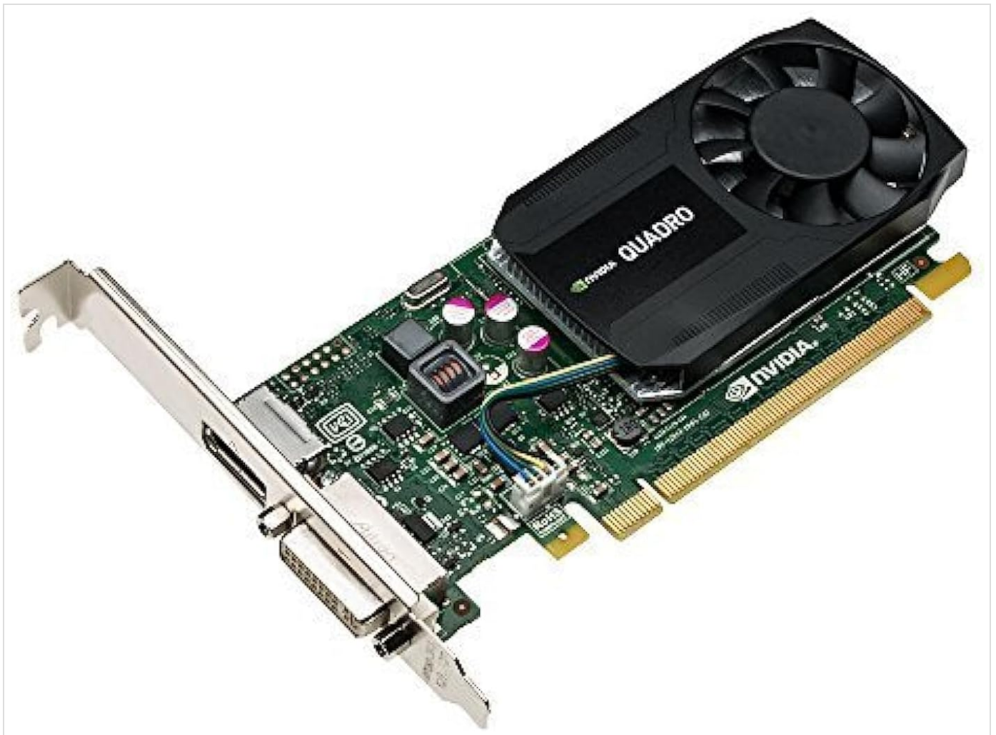
Figure 2.2.1: The PNY NVIDIA Quadro K620 Graphics Card. This image shows the full card, including the fan, heatsink, PCI Express connector, and display output ports (DisplayPort and DVI).
