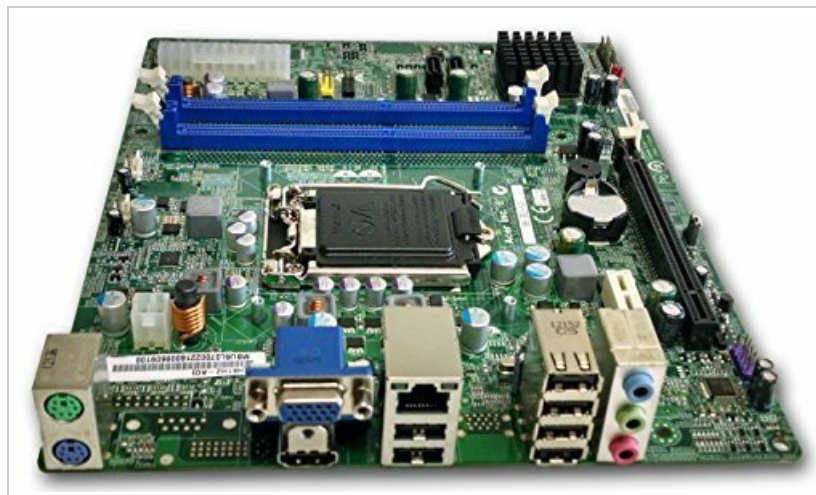
Figure 1: Overview of the Gateway SX2865 SFF Desktop Motherboard H61. This image displays the main components and layout of the motherboard, including the CPU socket, RAM slots, and various connectors.
