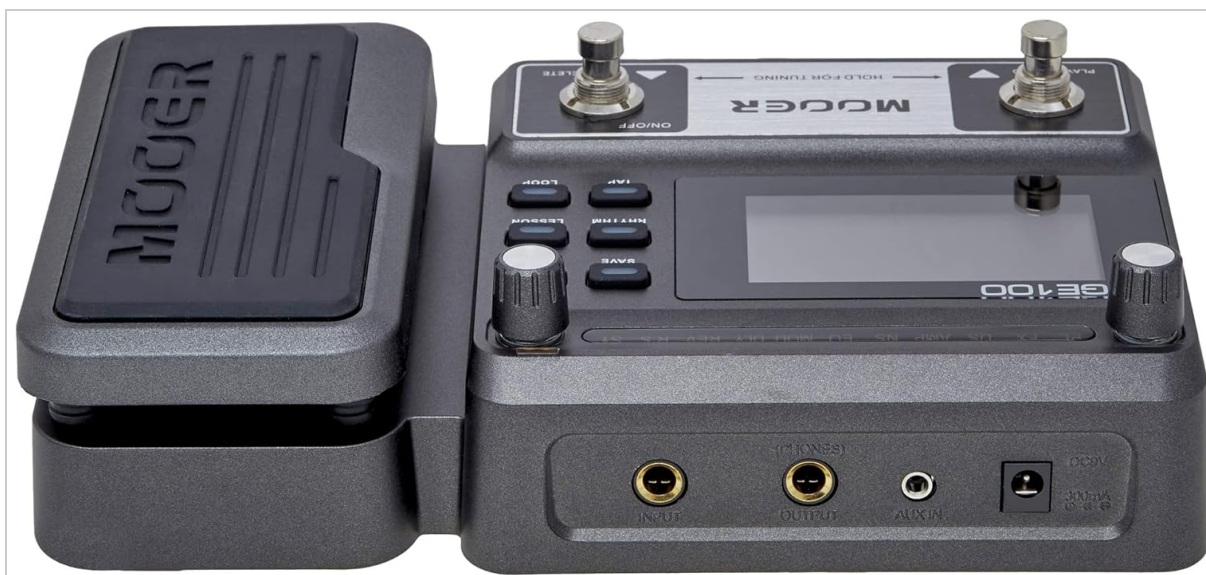
Figure 2: Rear panel of the MOOER GE100, illustrating the Input, Output, Aux In, Headphone, and DC In jacks.
