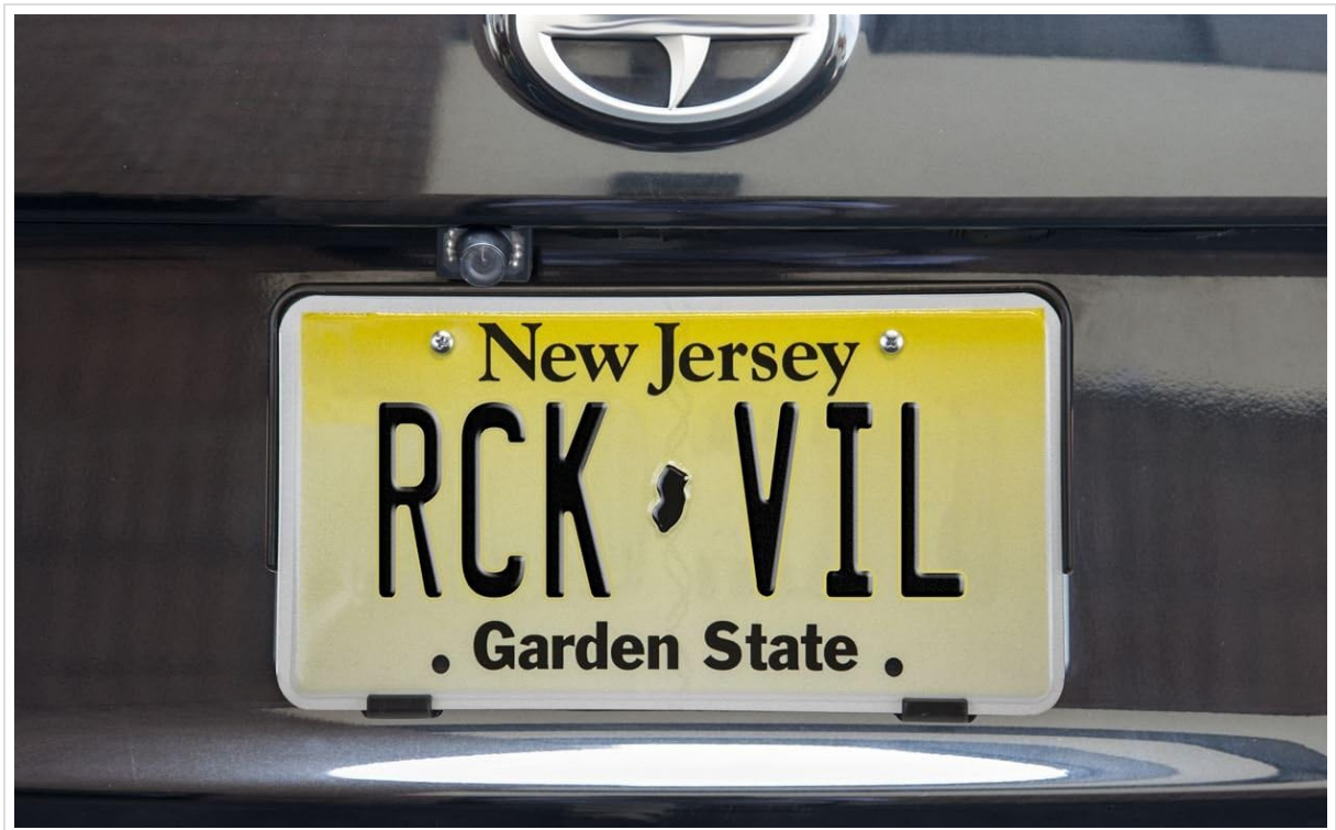
Image 2.4: Example of a backup camera installation on a vehicle.
