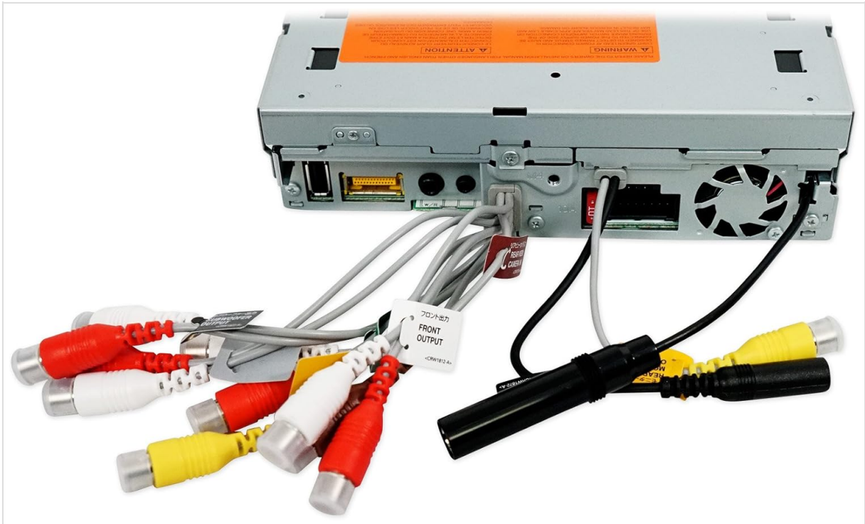
Image 2.2: Rear panel connections of the AVH-210EX receiver.
