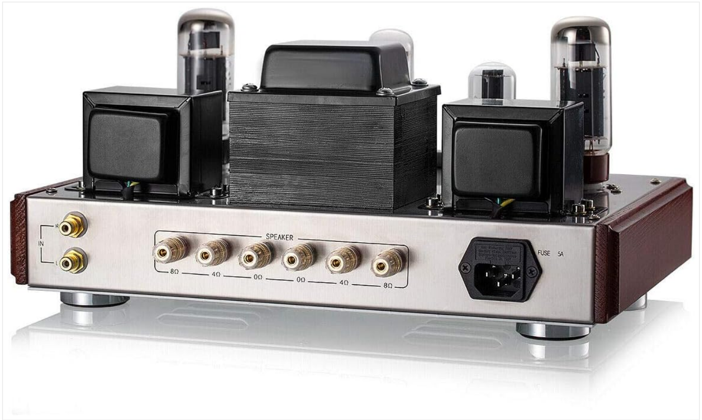
Image: Rear panel of the Nobsound EL34 amplifier, illustrating the RCA input jacks, speaker output terminals (4Ω and 8Ω options), and the power inlet with a 5A fuse holder.
