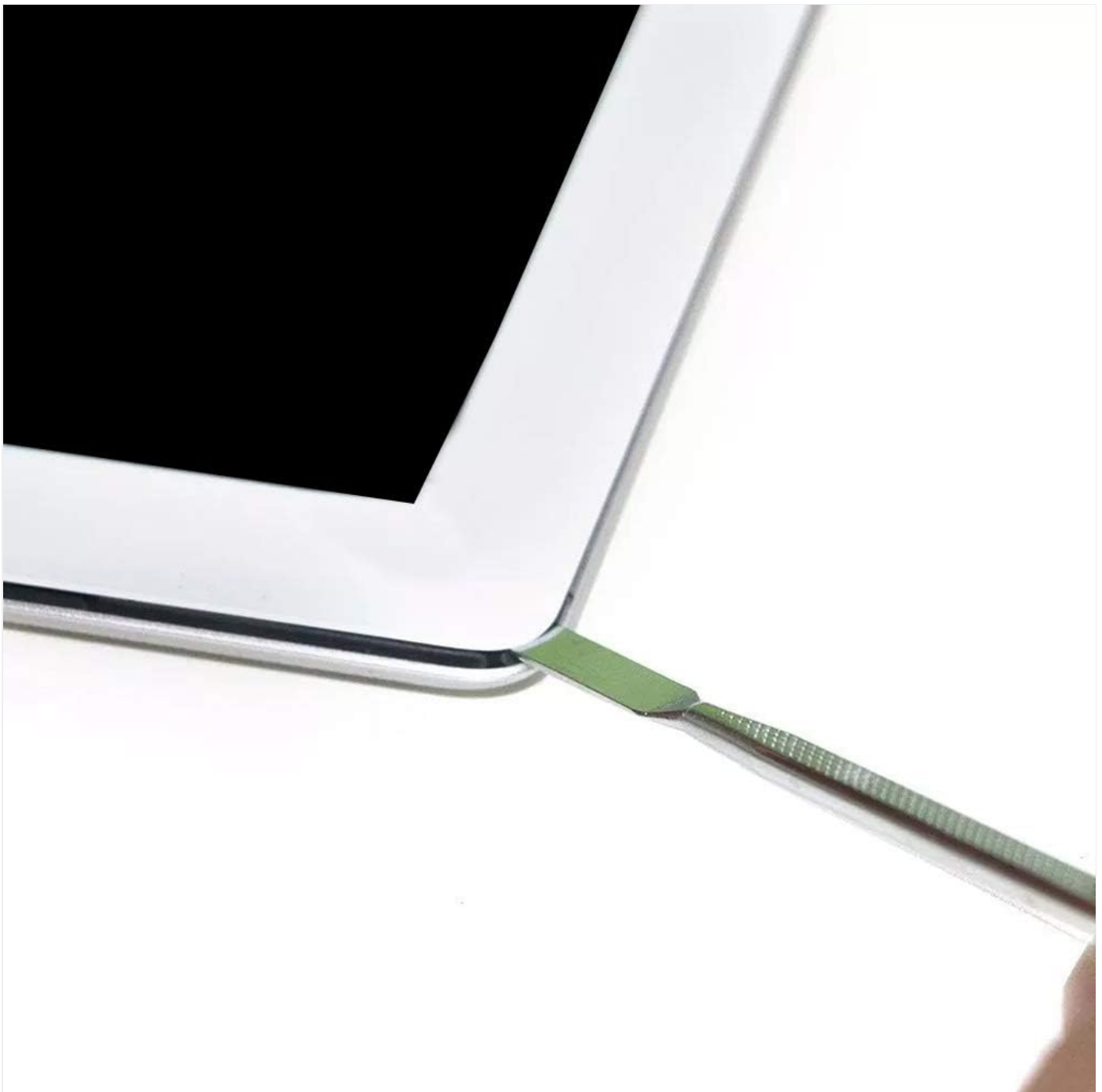
Figure 4: Carefully prying open the screen with a spudger.
