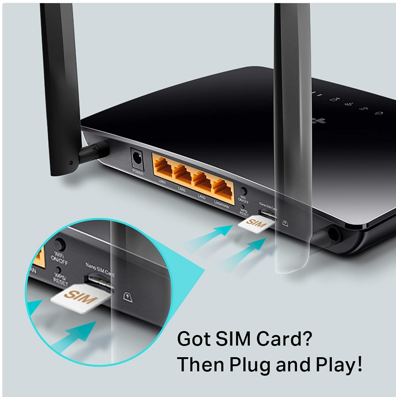
Figure 2: Proper insertion of the Nano SIM card.
