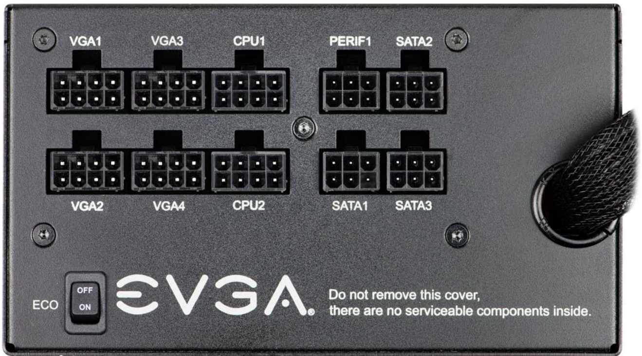
Image: A detailed view of the modular cable ports on the power supply, indicating connections for peripherals, SATA, CPU, and VGA.
