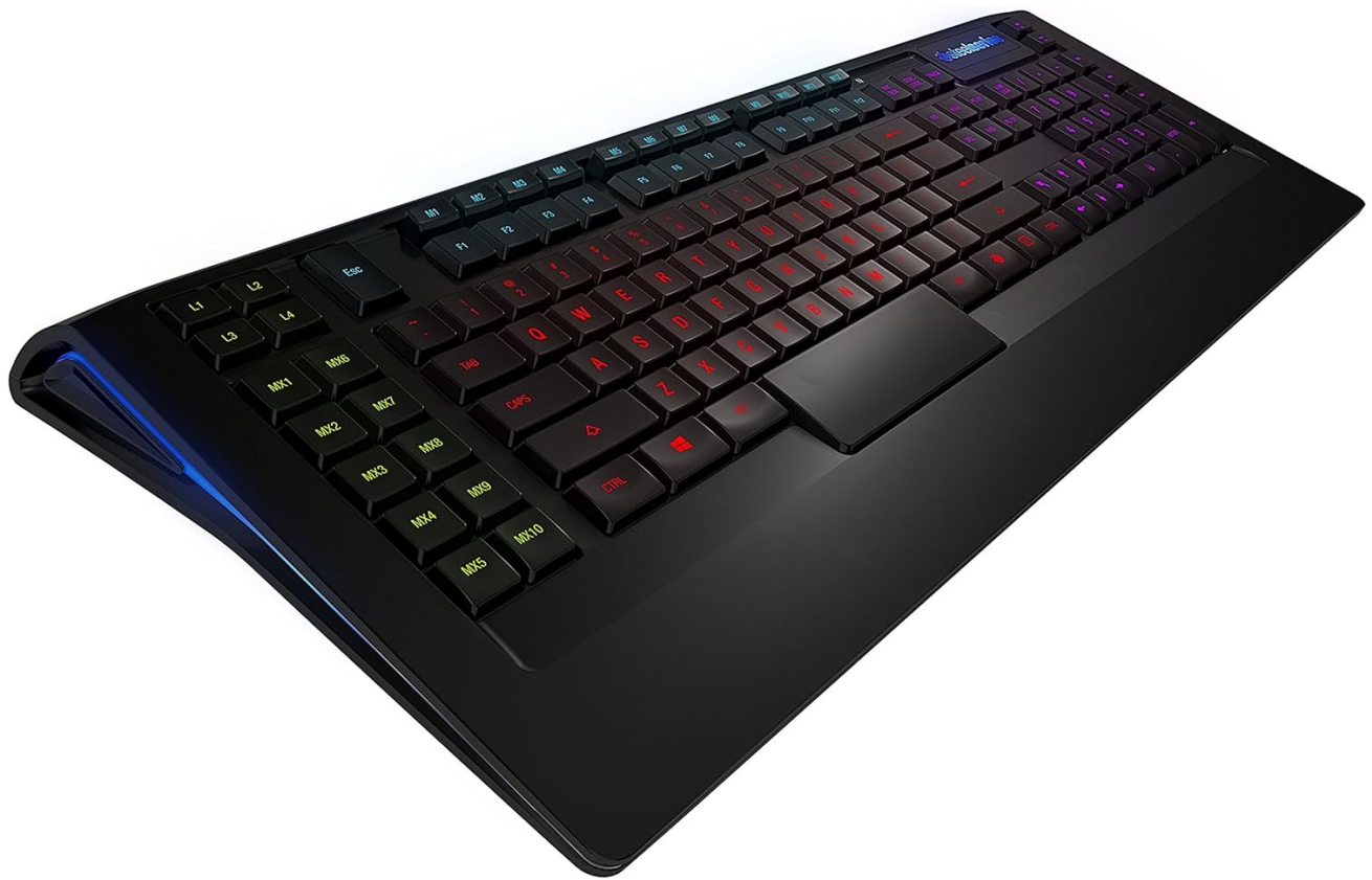
Image 4.1: Angled view showcasing the dedicated macro keys (M1-M10) and profile keys (L1-L4) on the left side of the keyboard.
