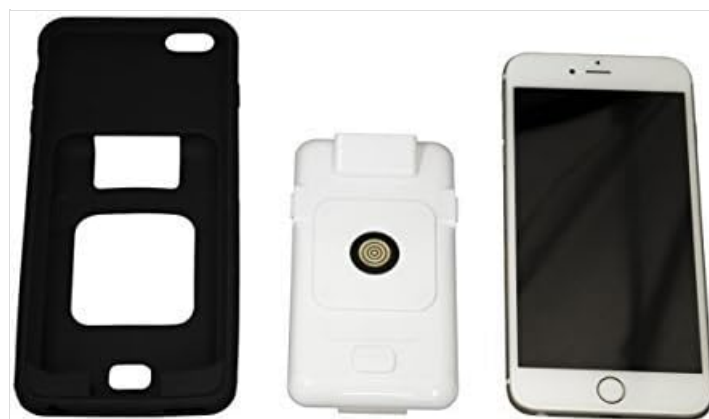
Figure 4.3: AsReader Components. This image shows the three main components of the AsReader system: a black protective case for the iPhone, the white AsReader 1D barcode sled module, and an iPhone. These components are shown separately before assembly.
