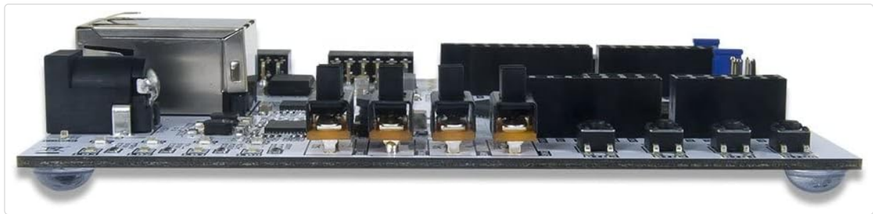
Figure 2.6: Side profile of the Arty A7-35T board, showcasing the various connectors such as the power input, USB port, and Ethernet port.
