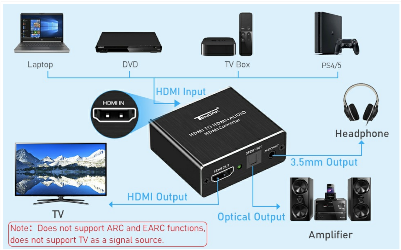
Image: Alternative connection diagram with various source and output devices.
