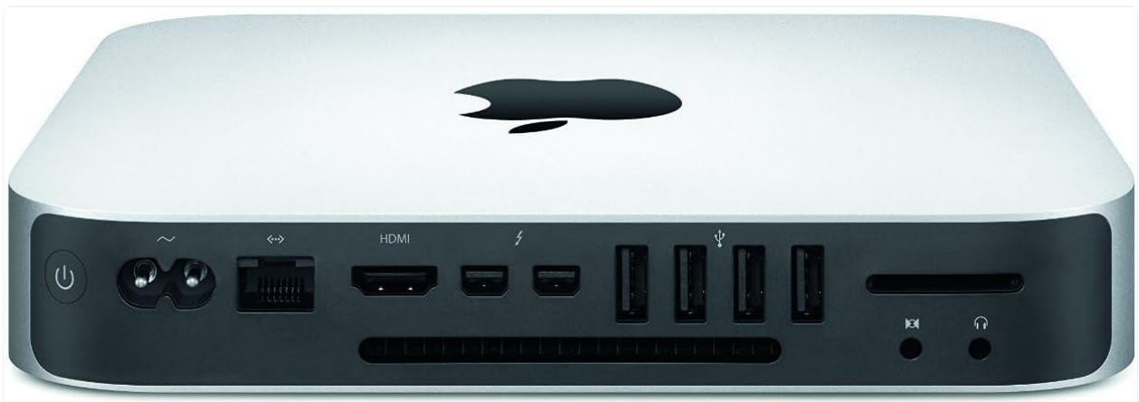
Figure 2: The rear panel of the Mac Mini, displaying the power input, Ethernet, HDMI, Thunderbolt, USB 3.0, SDXC card slot, and audio ports.
