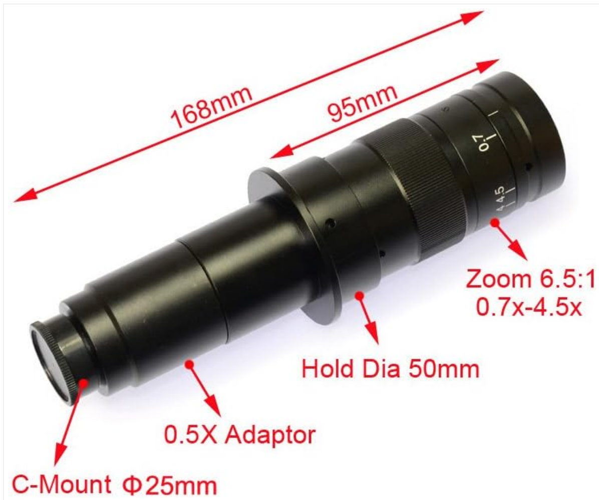
Figure 3.3: 180x C-Mount Lens Dimensions. Displays the lens with its various sections, including the 0.5X adaptor, zoom ratios (0.7-4.5X), and overall dimensions (168mm length, 50mm diameter).
