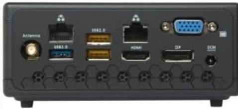
Image: Rear panel of the ZBOX CI323 Nano, featuring the Wi-Fi antenna connector, USB 3.0, USB 2.0, dual Gigabit Ethernet, HDMI, DisplayPort, VGA, and DC-in power input.
