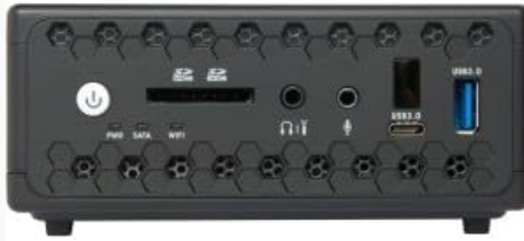
Image: Front panel of the ZBOX CI323 Nano, highlighting the power button, SD card reader, headphone and microphone jacks, a USB 3.0 port, and a USB Type-C port.
