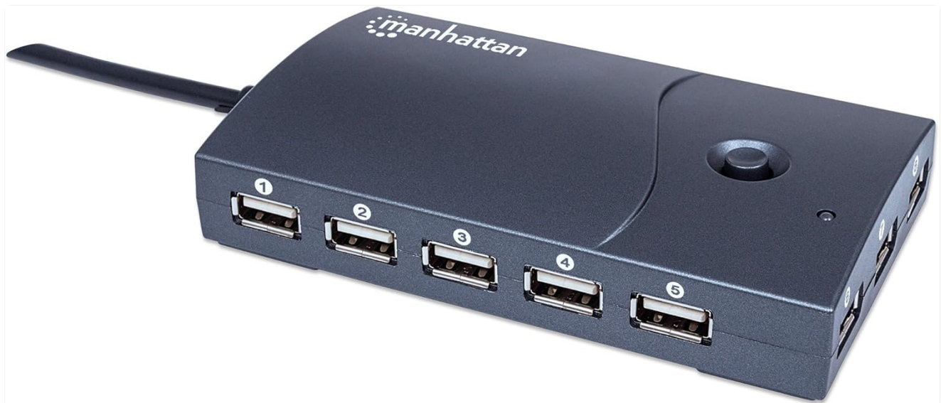
Image 1.1: Angled view of the Manhattan 13-Port USB 2.0 Hub, highlighting its compact design and multiple USB ports.
