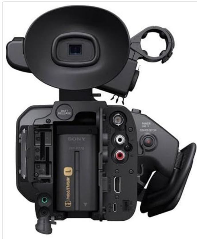
Figure 3.6: Rear view of the camcorder with the battery compartment open, showing the battery slot and various input/output ports.
