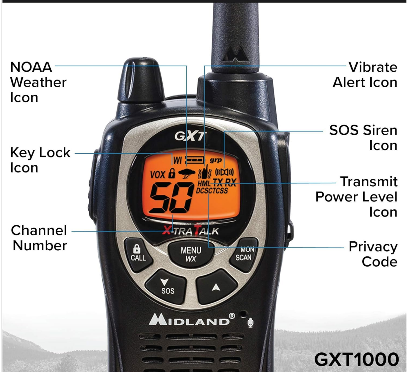
Image: Close-up of the Midland GXT1000VP4 radio display, showing labeled icons for NOAA Weather, Key Lock, Channel Number, Vibrate Alert, SOS Siren, Transmit Power Level, and Privacy Code.
