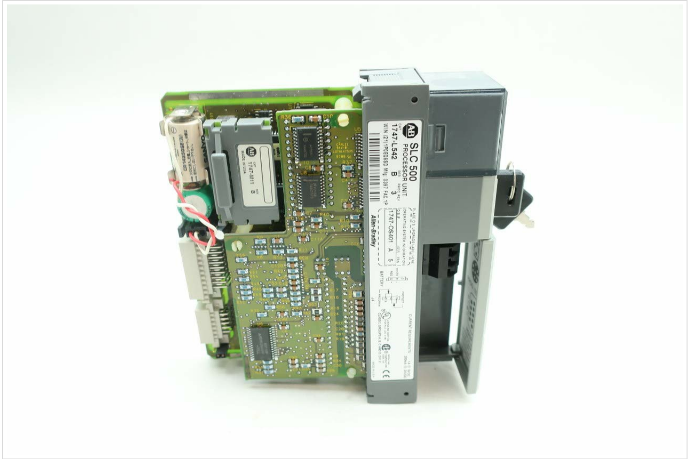
Figure 3: Side view revealing the internal circuit board and components, highlighting the modular design for maintenance and expansion.
