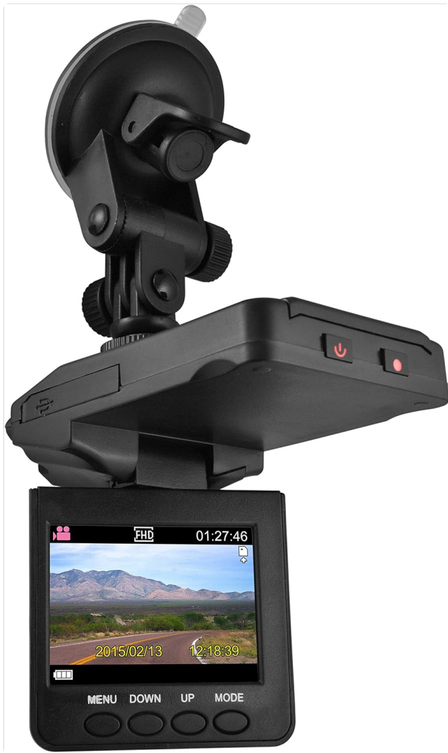
Figure 1: Front view of the Dash Cam with its display showing a recorded image and the suction cup mount attached.
