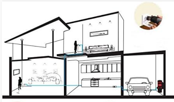
Image 3.2: Illustrative diagram of a typical central vacuum installation within a multi-story home, showing the main unit in the garage connected via piping to wall inlets throughout the house.
