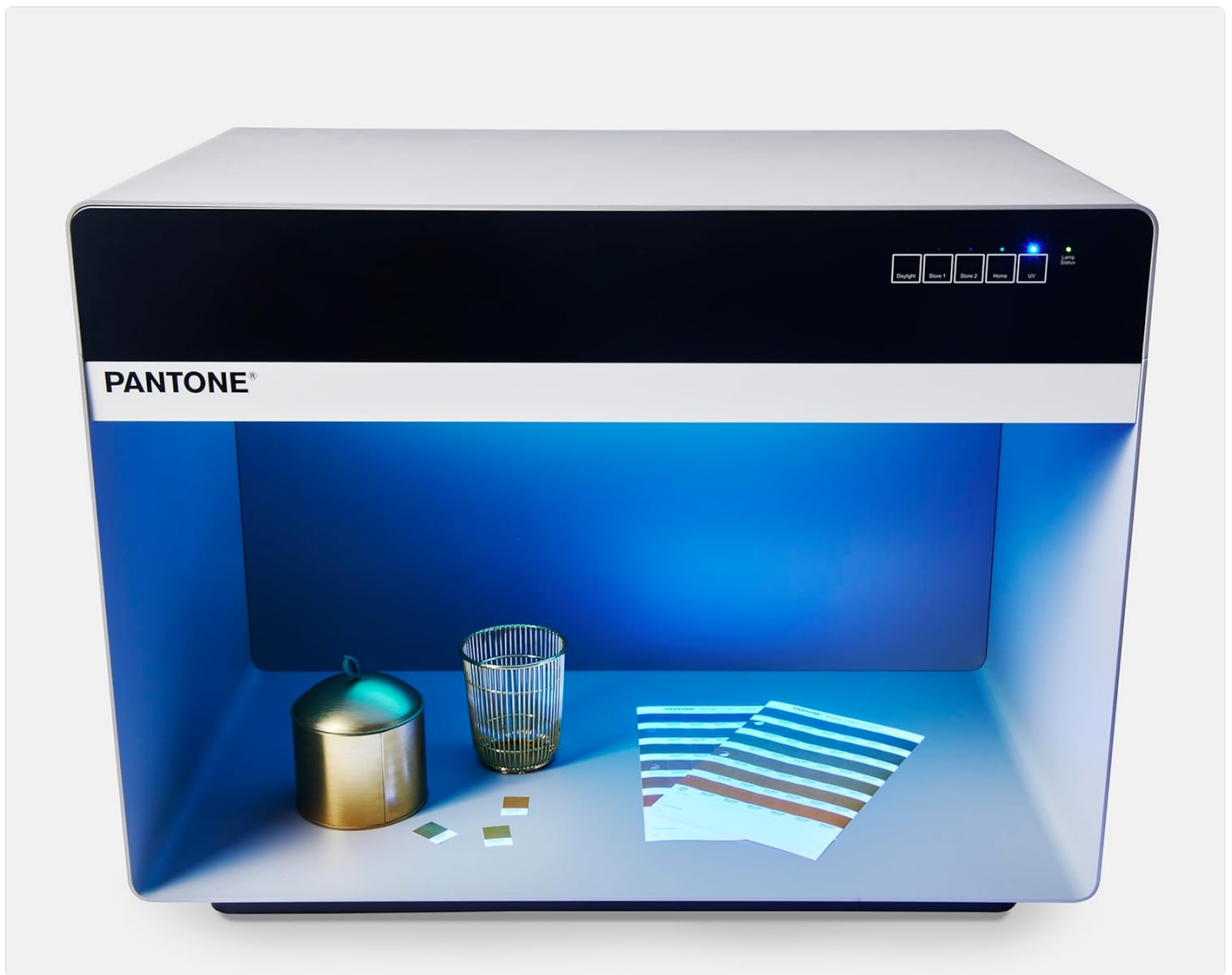
Image: The light booth under ultraviolet (UV) light, used to detect optical brighteners or fluorescence in materials.
