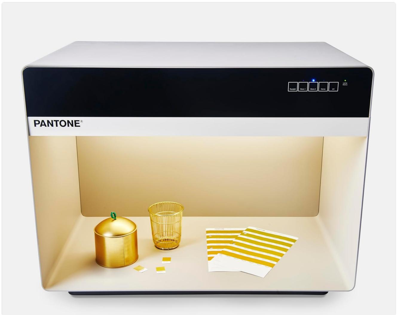
Image: The light booth under TL84 fluorescent light, representing another common commercial lighting scenario.
